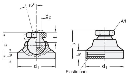
\* Complete with type index of the Levelling feet
